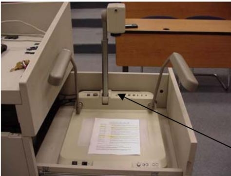
To activate the Elmo on the system, move the “Power” switch to the “on” position.
